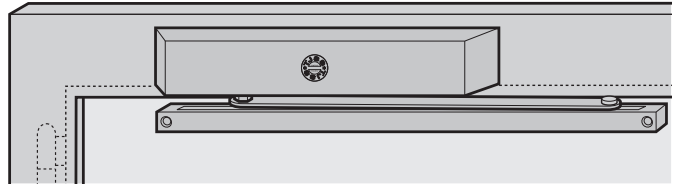
T46: push side top jamb installation
